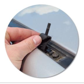
Hook clamps into the fixed points on the vehicle.
